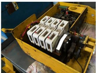
You can also see from that picture that the battery condition gauge is missing, it should be in the large round hole to the top right of the image— I am on the hunt for one of those currently as well.
